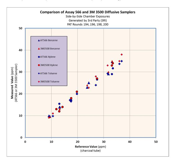
When measured Values for Diffusive Samplers were plotted versus the Reference Values for each exposure, the correlation co-efficients for each sampler for all three analytes were 0.98 or better.
