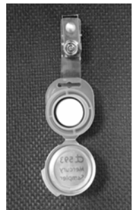
Monitor with Filter in place
